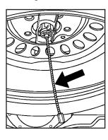
Check under the vehicle to see if the cable is visible. If it is not visible, see Secondary Latch System on page 5-82.
